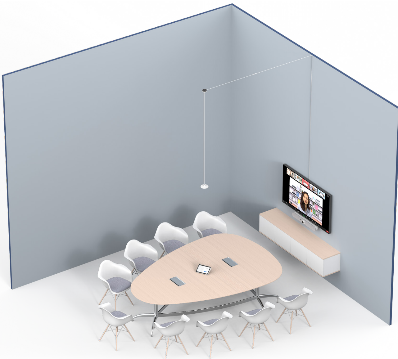
Figure 1 - A Mic Pod with Pendant Mount. In this image, the mic pod cable is connected to a Mic Pod Extension Cable, which is connected to Rally Bar Mini under the TV. Note: Image not to scale.
